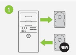
If you are replacing a hard drive, install the new one according to the instructions in your computer's user guide. When replacing the drive, ensure that it is as large in capacity as the original drive. Otherwise, if you are recovering your data to your current drive, move on to step 2.
